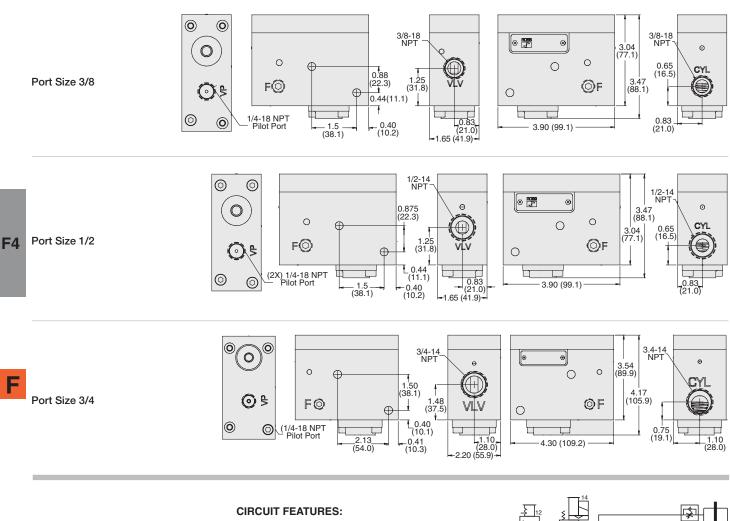
Trapped pressure between check valve and cylinder is exhausted when the manual relief button is pressed.
