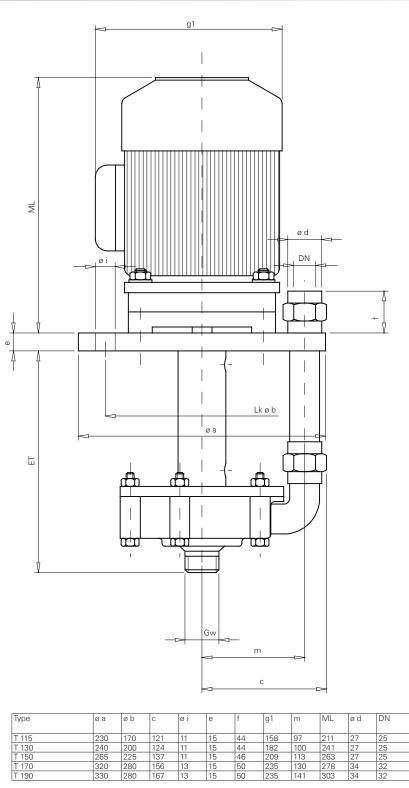
The dimensions of the motors refer to three-phase standard motors.
