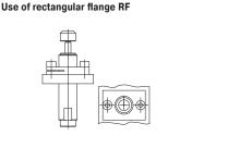
Mounting of damper in borehole with two locknuts
