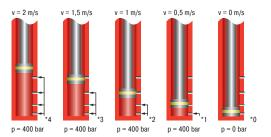
\* The load velocity reduces continuously as you travel through the stroke due to the reduction in the number of metering orifices (\*) in action. The internal pressure remains essentially constant and thus the Force vs. stroke curve remains linear.
