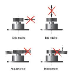
No axial or radial forces may be introduced via the shaft. The rotary axis was not designed for side loading (see diagrams).
