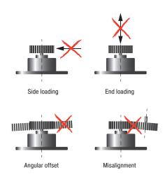
rotary axis was not designed for side loading (see diagrams).
