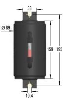
AO6 Oil capacity 2,600 cm<sup>3</sup> Material: Steel
