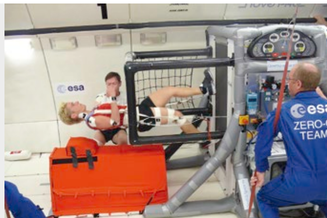
TUBUS are used to protect a fitness machine in zero gravity QinetiQ Space nv, BE9150 Kruibeke, Belgium
