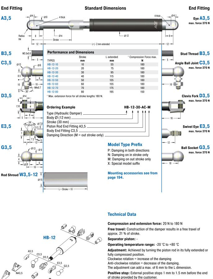
Material: Outer body: Coated steel; Piston rod: Stainless steel (1.4301/1.4305, AISI 304/303); End fittings: Zinc plated steel
