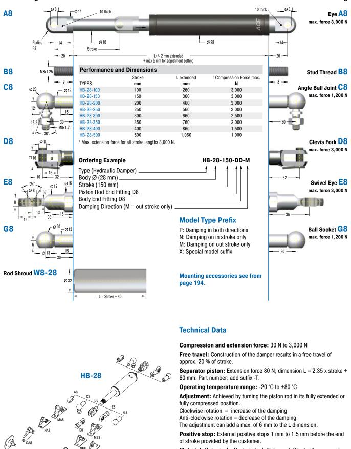
**Material:** Outer body: Coated steel; Piston rod: Steel with wear-resistant coating; End fittings: Zinc plated steel
